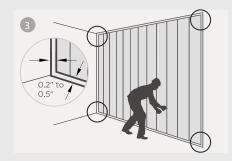
Leave a 0.2-0.4" gap around the perimeter. Avoid direct floor installation; mantain at least 0.4" gap to prevent fluid contact.
