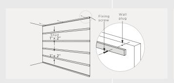
For leveling and insulation, cover walls with MDF's or wood furring strips every 16". Do not install on irregular or humid walls (moisture content should be below 12%). It is not recommended to install directly on walls with irregularities or that release humidity.
