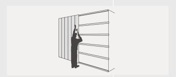
Install additional wood panels using a rubber hammer or wooden block. Avoid striking the shiplap edge directly with the hammer as this could cause damage.
