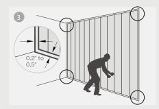
Leave a 0.2-0.4" gap around the perimeter. Avoid direct floor installation; mantain at least 0.4" gap to prevent fluid contact.
