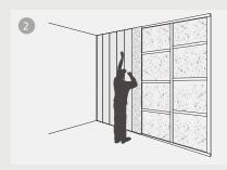
Attach panels with high elasticity adhesive. For extra hold, use 0.13" flat head screws or finishing nails at the edges of fluted panels or on the melamine surface of fluted panels.
