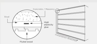
Install wood panels from left to right. Ensure the first piece is level, then secure with adhesive. For added stability, use 0.13" flat head screws of finishing nails at the edges or on the Melamine surface.
